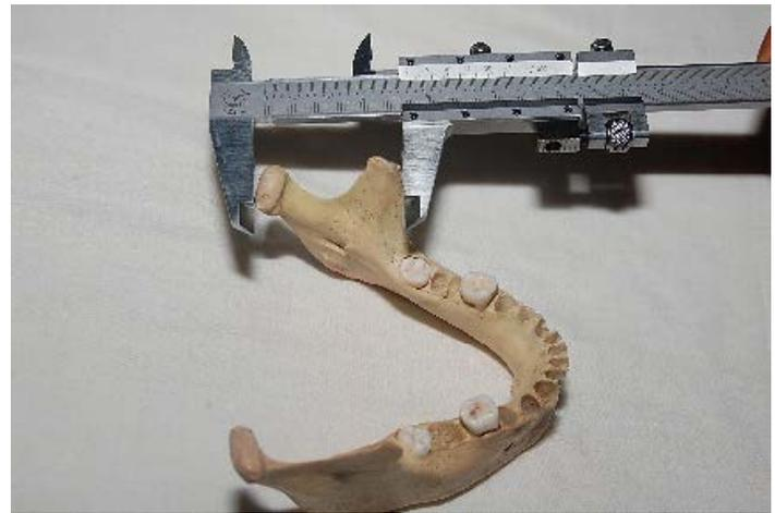
**Fig-2:** Maximum ramus breadth measured using sliding caliper
